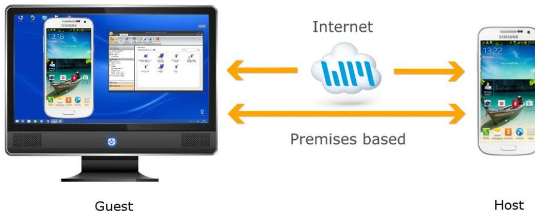
The security mechanism in the Android operating protects access to certain API functions so only authorized access is allowed. In order to capture the screen and inject keyboard and touch events the Remote Control App needs access to such functions.
